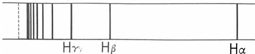
**HYDROGEN SPECTRUM** expresses the behavior of a fundamental constituent of matter, the electron. Shown above is a part of the Balmer series of spectral lines, which are in the visible light range. Each line is the result of a change in energy of the atom's electron.
