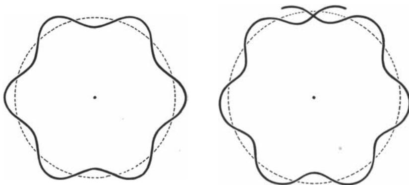
**WAVE MECHANICS** sees the electron not as a point mass, but as a standing wave washing to and fro in the atom. Some modes of vibration are possible (*left*), while others are not (*right*). The possible modes correspond exactly to the Bohr theory's possible energy levels.
