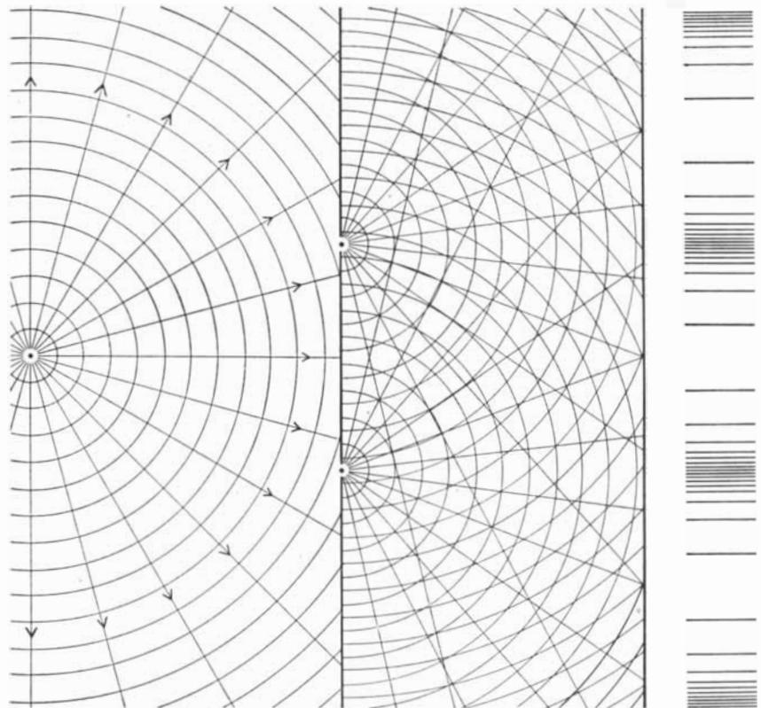
**INTERFERENCE** is also evidence of waves. Its characteristic pattern is formed when rays interact. For light waves the pattern shows up as bright and dark bands on a screen (*right*).
