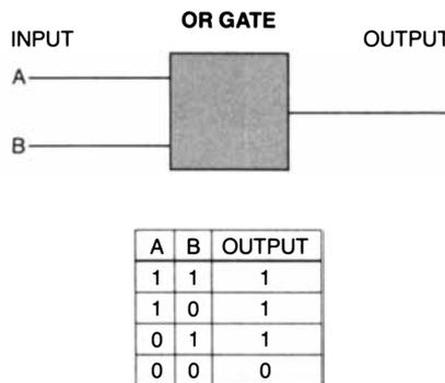
**CONVENTIONAL LOGIC GATES** dissipate energy because they discard information. For example, if the output of an *and* gate is 0, there is no way to deduce what the input was.
